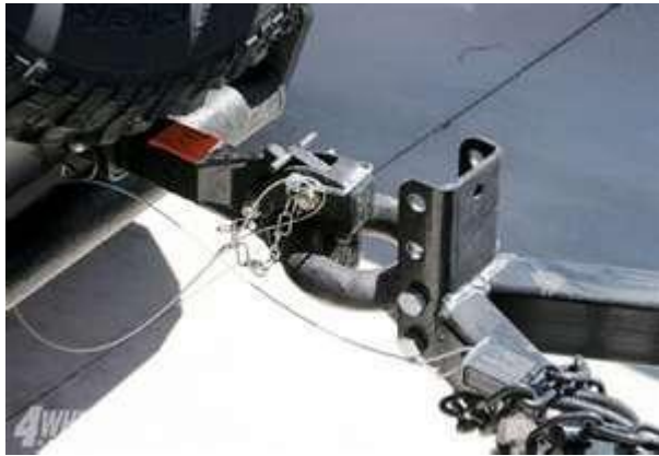
Trailer with Ball-hitch Coupler or Pintle Ring
