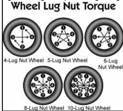
Figure 6-1 Lug nut sequence of tightening
