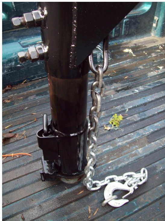
Gooseneck Ball Receiver and Height Adjustment
